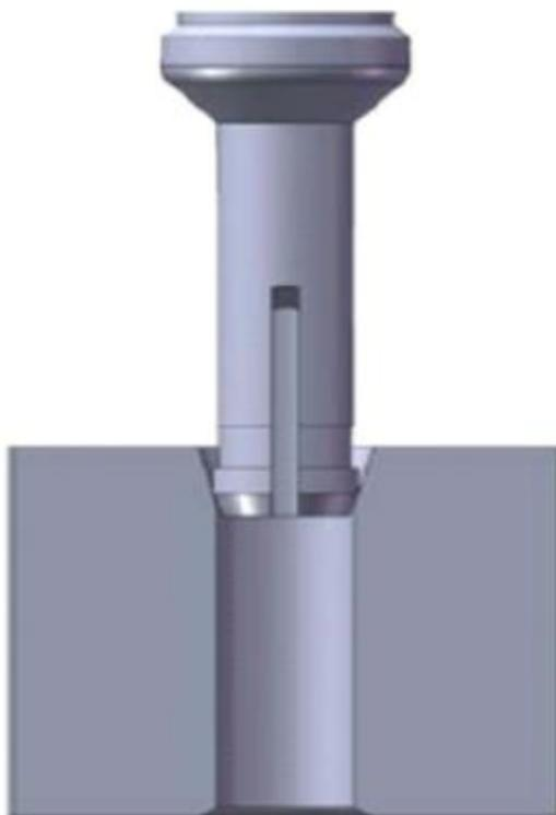
**Figure 14 – Collet unit of fuel element**
