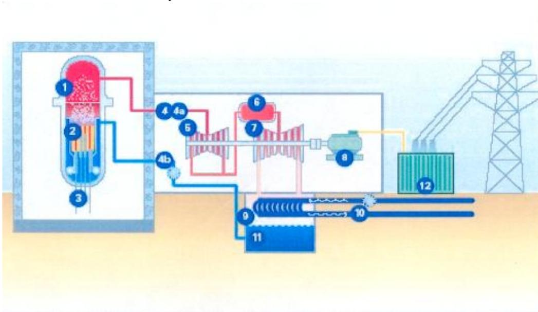
(1) reactor, (2) core, (3) absorbing rods, (4) primary cooling circuit, (4a) steam for turbine, (4b) water for reactor, (5) high-pressure cylinder, (6) steam superheater, (7) low-pressure cylinder, (8) generator, (9) condenser, (10) cooling water circuit, (11) condensate, (12) transformer.
