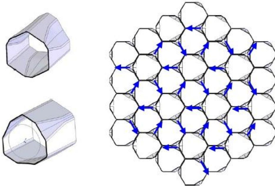
**Figure 21 – Cells and a part of mixing grid of “cyclone” type.**
