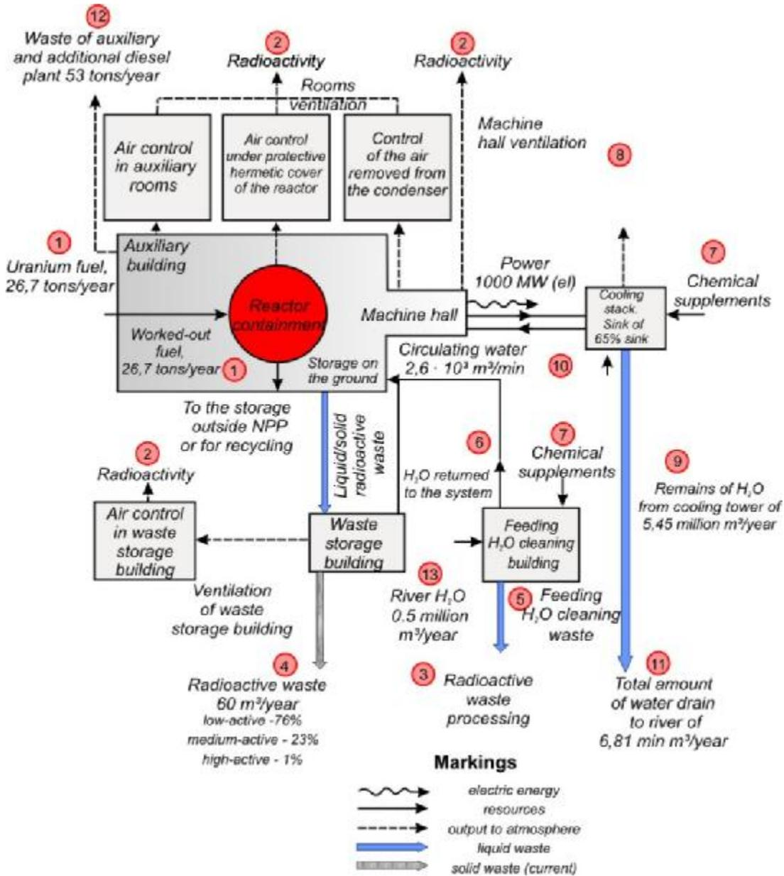
Figure 33 – PWR reactor Units of impact on the environment
