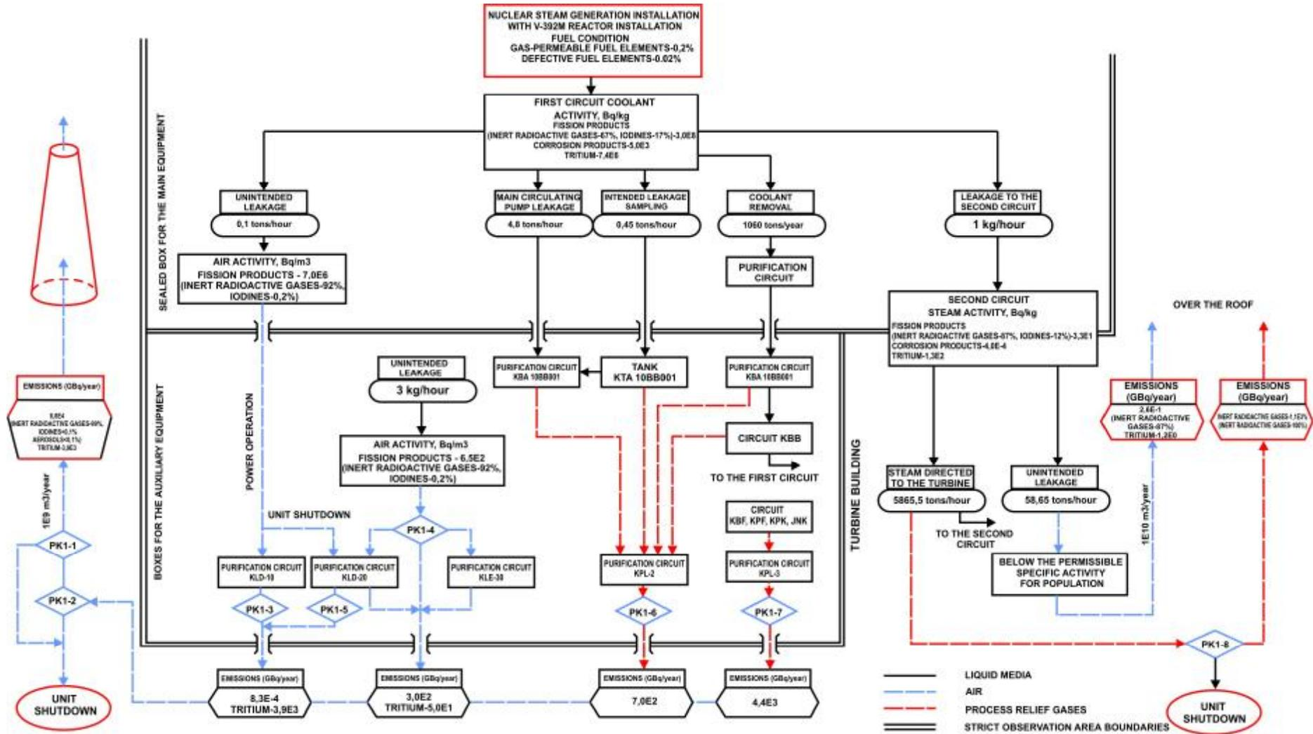
Figure 35 – Balance diagram of possible output of radioactive gases and aerosols into the atmosphere
