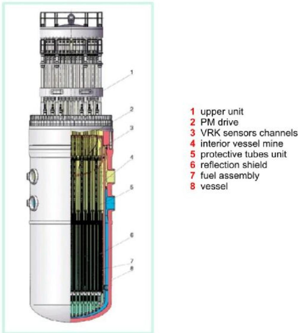
**Figure 9 – Longitudinal plan of the reactor**
