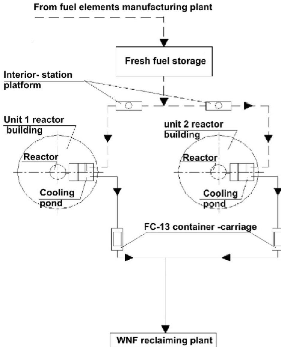
Figure 37 - Functional diagram of nuclear fuel handling
