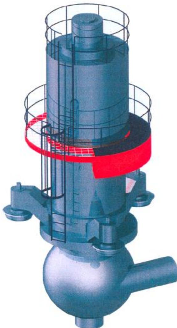
**Figure 24 – Main circulating aggregate**
