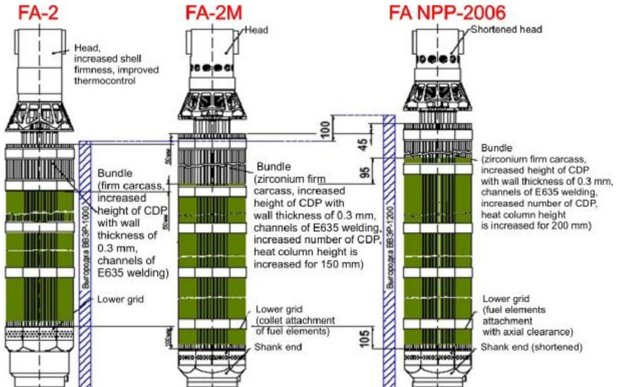
**Figure 11 – FA evolution in lengthening of fuel column**
