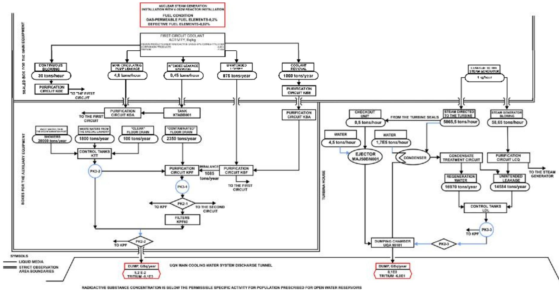
Figure 36 – Output of radioactive substances into the environment with liquid non-radioactive dumps at plant operation in normal mode
