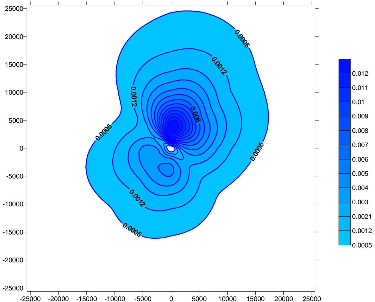
**Figure 34 – Distribution of calculated increases of ground specific humidity (g/kg) around Nizhniy Novgorod NPP cooling towers. Point with coordinates (0.0) is the place where colling stacks are sitiated. Distance from the cooling towers (m) to the north and east is positive, to the south and west is negative**
