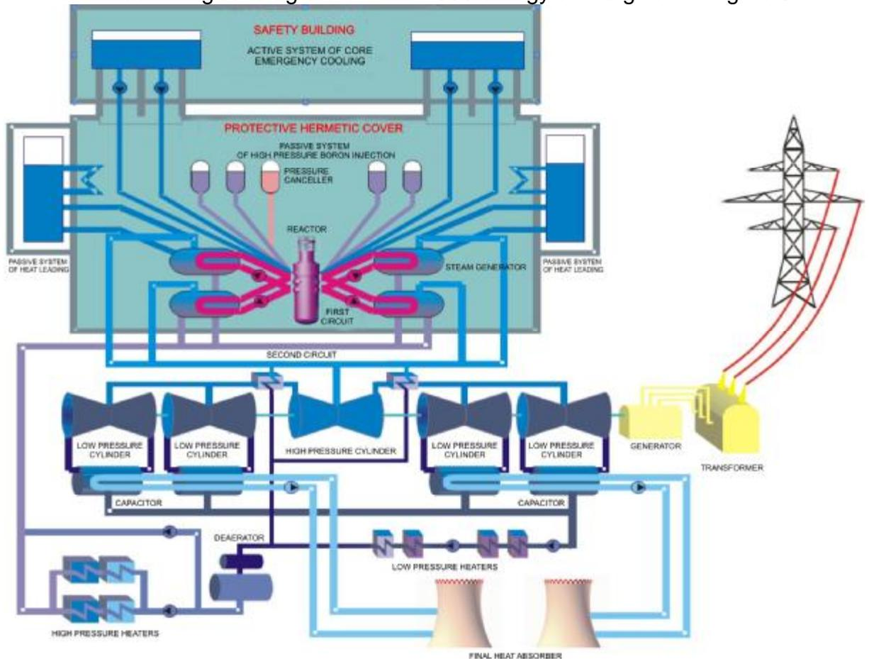
Figure 8 – Functional technological diagram
