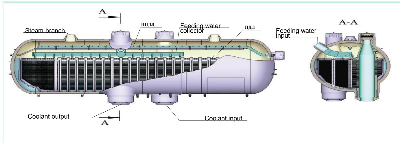
Figure 23 – Longitudinal section of a steam generator
