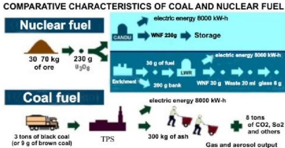
**Figure 2 – Comparison of types of fuel and waste at burning**
