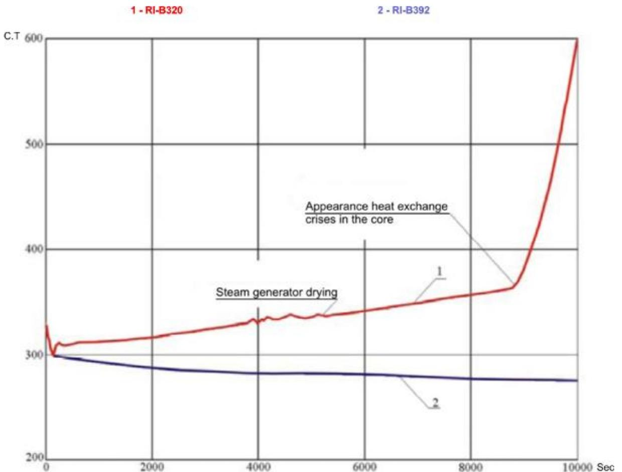
**Figure 29 – Maximum temperature of fuel element cover at full loss of alternative current sources**
