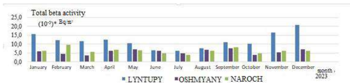
Figure 9.2 – Monthly averages of total beta activity in samples of aerosols from the surface layer of the atmosphere at observation points located in the area of impact of the Belarusian NPP for 2023
