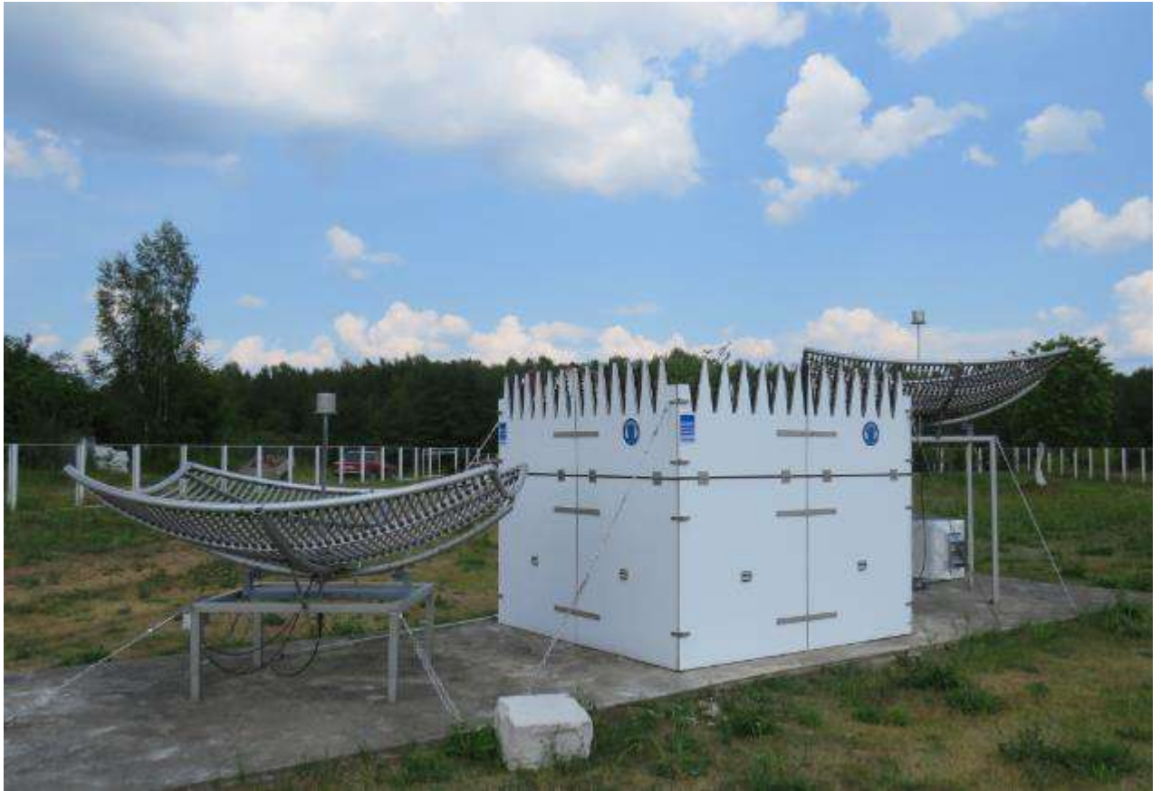
Figure 8.17- SODAR measuring complex
